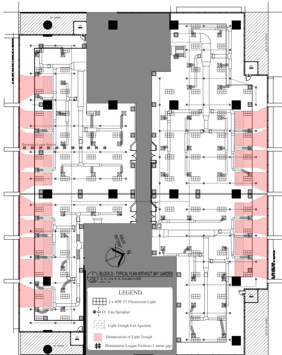
Figure 10 Ceiling layout plan of a typical office level with DT location demarcated
